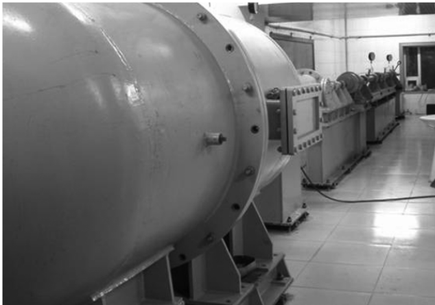
Fig. 2 The two-stage light gas gun for impact experiment.
